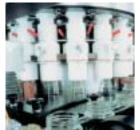
Dosing head made of ERTALYTE® TX in bottle & glass filling equipment
